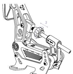
You can also set the spring pre-load (and also the return speed) using the supplied HEX4mm L key on the screw in the front of the pedal.
