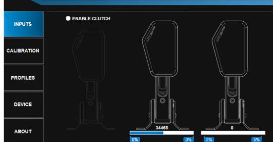
In this case, by clicking on the "CALIBRATE" section, you will be able to calibrate them. Then simply clicking "CALIBRATE" once again will make the RAW values of the pedals appear.
