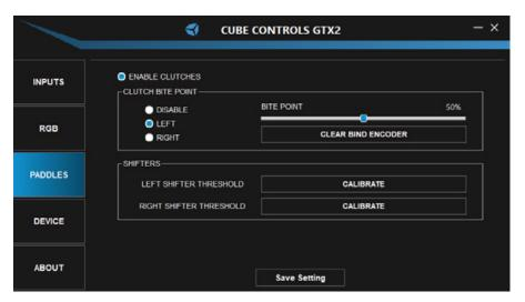
On the PADDLES page, you have the CLUTCHES section and the SHIFTERS section. In the CLUTCHES section, you can enable/disable the clutches and the Bite Point. For the Bite Point, you will also be able to select the Slave Clutch to be the Left or the Right one and then limit the percentage for it. In the SHIFTERS section, you will be able to Calibrate automatically the shifters to ensure full compatibility!
