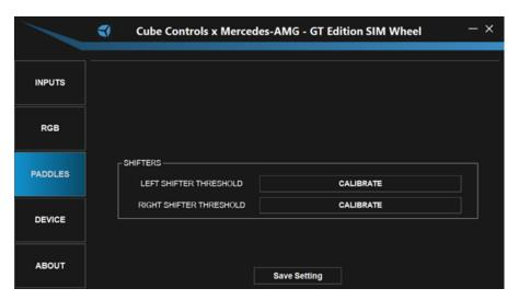
On the PADDLES page, you have the CLUTCHES section and the SHIFTERS section. In the CLUTCHES section, you can enable/disable the clutches and the Bite Point. For the Bite Point, you will also be able to select the Slave Clutch to be the Left or the Right one and then limit the percentage for it- and also bind it to an encoder of the wheel to modify the bite point on the fly! In the SHIFTERS section, you will be able to Calibrate automatically the shifters to ensure full compatibility!
