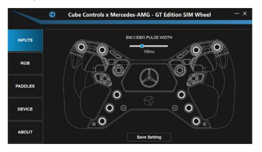
On the INPUTS page, you can check the correct functionality of every button and encoder present in your wheel, modify the Encoder Pulse Width.
