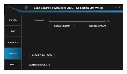
On the DEVICE page, you can update your steering wheel's Firmware, Factory Reset your wheel and also check your Battery Status (only when on BLE connection).
