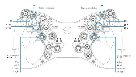
The **POV** switches/funky switches/joysticks directions (up, down, left, right) are meant to work only if a "clicky" sound feedback occurs. Therefore there's no risk to press the direction and accidentally enable the centre click button.
