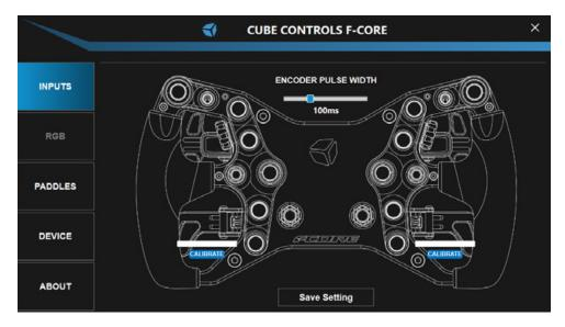
On the INPUTS page, you can check the correct functionality of every button and encoder present in your wheel, modify the Encoder Pulse Width and calibrate the Clutches (if present).
