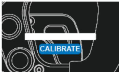
In this case, clicking on “CALIBRATE” will make the RAW values of the clutch appear. Pressing now the clutch full-course will make the system set the correct minimum and maximum values.
