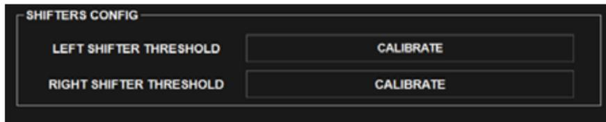
The **CALIBRATE** button will be replaced by the message “**press and hold the left shifter then click me**”.
