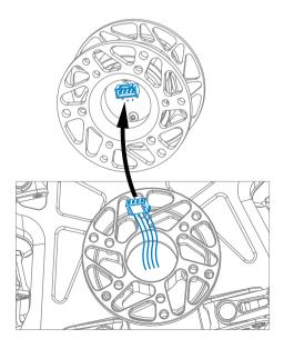
Now carefully align the QRX body with the steering wheel hub making sure to not pinch the cables between it and the wheel hub, and secure it using the three torx screws provided, by using the non-threaded holes as in the drawing:
