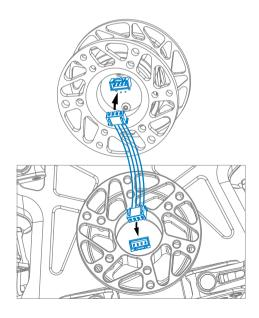
The 4-pin wire connector can be installed directly on the QRX's main body on the mating female socket.
