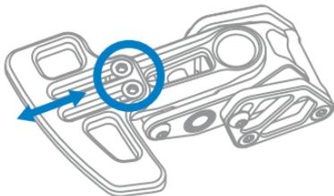
Reach can be adjusted by slightly loosening the screw highlighted as the right picture and the one on the opposite side of the shifter as pointed by the small arrow, then rotating the lever body upwards/downwards. You may need to apply a bit of force. Make sure to firmly secure the screw once the adjustment has been made.
